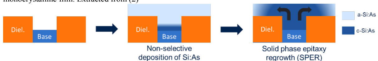
Figure 1. Schematics of the non-selective deposition of Si:As to fabricate the emitters of bipolar transistors. The combination of amorphous deposition (light blue) on dielectrics (orange) and SPER generates a fully monocrystalline film. Extracted from (2)
